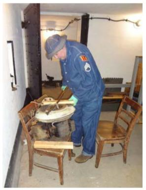
This very heavy assembly, probably over 100 pounds, had to be taken apart to clean and inspect the parts. The motor, which is still in working order, is 2-Phase Direct Current (DC), and AGFA members are brain-storming on how to best utilize this
