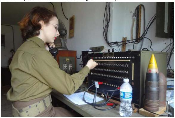
Always of great interest to visitors is our Wind Component Indicator. This device, built in 1906, was used through WWII to determine the effect that varying wind speeds and directions would have upon the flight of a projectile.
